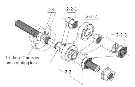
2-2 Set up the arrangement of freewheel side orderly, reference (FL) the original width from hub side. piled up with suit thickness spacer or washers when necessary.
